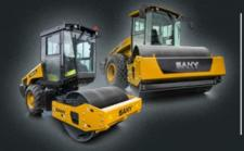
SINGLE DRUM COMPACTORS SSR80C-8 SSR120C-8 Engine YANMAR / CUMMINS Centrifugal force 132 kN / 280 kN Working width 1 676 mm / 2130 mm Weight 7 330 kg / 12,000 kg
